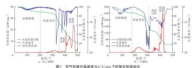
Fig.2 Oxidation phase division at temperature rise rate of 6 °C/min in air environment
