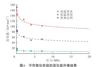
Fig.6 Extrapolation results of activation energy at different oxidation stages
