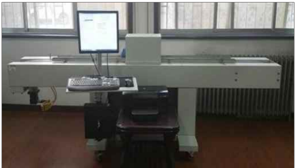
a.岩心地面伽马能谱测量仪
